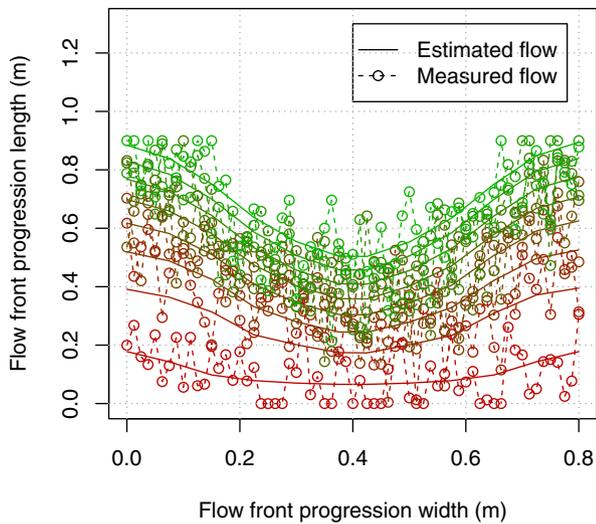
Fig. 7. The estimated flow-front with 12 lines (states), sampling frequency = 0.25 Hz, and the measurement noise  $\sigma = 0.1$ . The dot-dashed lines indicate the measurements from the true system and the solid lines indicate the estimated flow-front. The line colour changes gradually from red at the first time instance to green at the last time instance.
