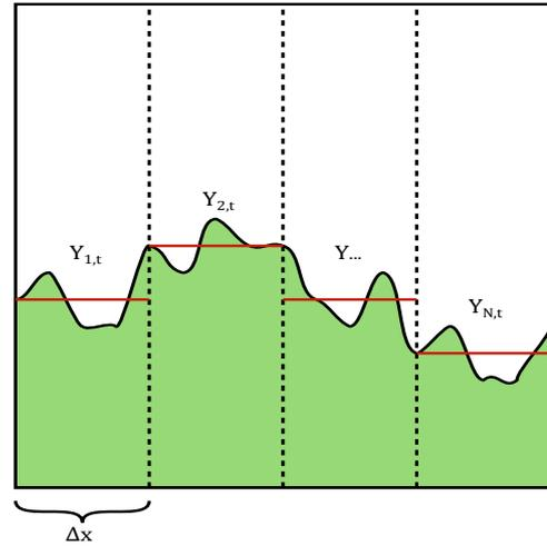
Fig. 4. A pictorial representation, how the flow-front is approximated using the coupled SDEs. The red line shows the domain of spatial dimension  $x$  which is approximated using a SDE, whereas the dotted vertical lines show the points of discretisation for the spatial dimension  $x$ .
