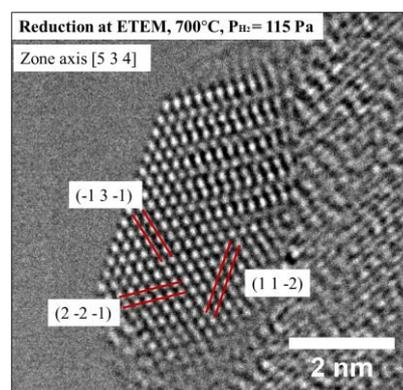
**Figure 1.** High-resolution TEM image of a Ni<sub>5</sub>Ga<sub>3</sub> ( $\delta$ -phase) nanoparticle acquired in the ETEM under reduction conditions (700 °C, 1.15 mbar H<sub>2</sub>).
