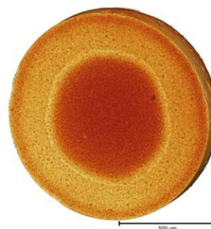
**Figure 2.** Computed X-ray micro tomography image of reconstructed 3D volume of the Ni-Fe catalyst. The  $\gamma$ -Al<sub>2</sub>O<sub>3</sub> sphere is approx. 1 mm in diameter.
