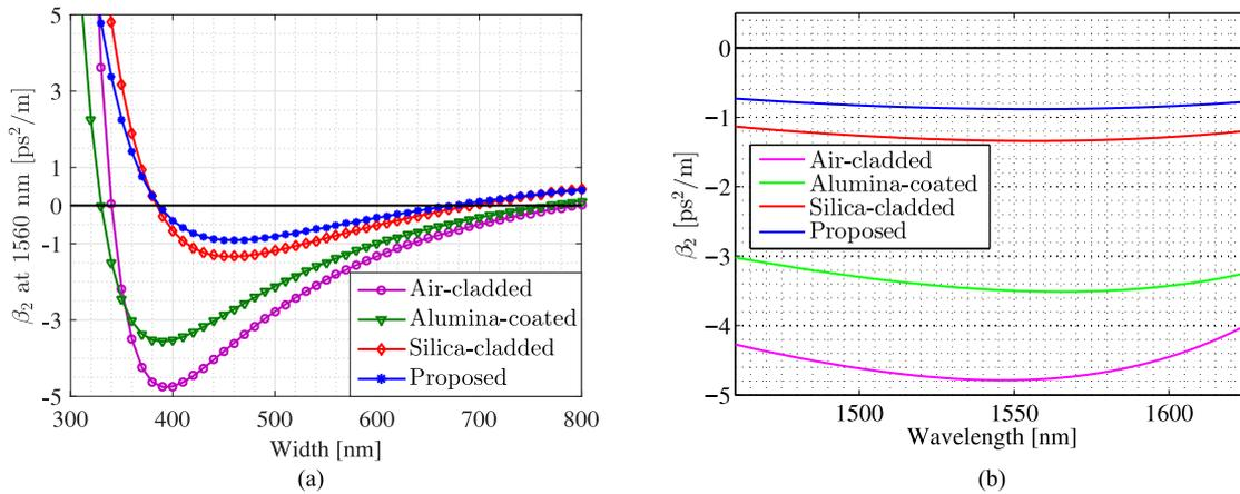
Fig. 2. (a)  $\beta_2$  at 1560 nm versus core width  $W$  for the air-cladded structure (magenta circles), the alumina-coated structure (green triangles), the silica-cladded structure (red diamonds), and the proposed structure (blue asterisks). (b)  $\beta_2$  versus wavelength for the air-cladded structure (magenta), the alumina-coated structure (green) when  $W = 390$  nm, and for the silica-cladded structure (red), the proposed structure (blue) when  $W = 460$  nm.
