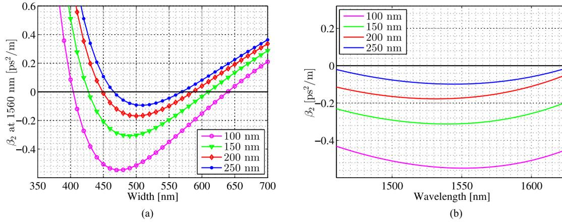
Fig. 3. (a)  $\beta_2$  at 1560 nm versus  $W$  in the proposed structure for different coating thickness  $T$  of 100 nm (magenta circles), 150 nm (green triangles), 200 nm (red diamonds), and 250 nm (blue asterisks). (b)  $\beta_2$  versus wavelength in the proposed structure when  $T = 100$  nm and  $W = 470$  nm (magenta),  $T = 150$  nm and  $W = 480$  nm (green),  $T = 200$  nm and  $W = 490$  nm (red),  $T = 250$  nm and  $W = 510$  nm (blue).
