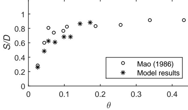
**FIG. 4. Equilibrium scour depth versus Shields parameter for both experimental, data taken from Mao (1986), with  $\theta \approx 0.03 - 0.43$  and  $D = 0.05 - 0.1$  m, and modelled, with  $\theta = 0.026-0.172$  and  $D = 0.03$  m.**
