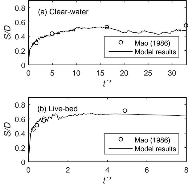
**FIG. 2. Comparison of modelled and experimental non-dimensional scour depth. Experimental data taken from Mao (1986). (a) Clear-water, with  $\theta = 0.048$  and  $D = 0.1$  m in the experiments, and  $\theta = 0.044$  and  $D = 0.03$  m in the model results. (b) Live-bed, with  $\theta = 0.098$  and  $D = 0.1$  m in the experiments, and  $\theta = 0.098$  and  $D = 0.03$  m in the model results.**
