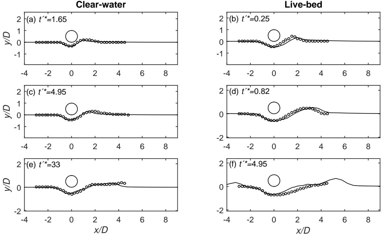
**FIG. 3. Comparison of modelled (circles) and experimental (lines) scour profiles at different times. Experimental data taken from Mao (1986). Left, clear-water, with  $\theta = 0.048$  and  $D = 0.1$  m in the experiments, and  $\theta = 0.044$  and  $D = 0.03$  m in the model results. Right, live-bed, with  $\theta = 0.098$  and  $D = 0.1$  m in the experiments, and  $\theta = 0.098$  and  $D = 0.03$  m in the model results.**
