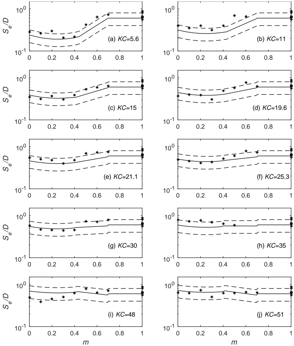
**FIG. 8. Equilibrium scour depths. Solid lines: Empirical expression (13) from Sumer and Fredsøe (1996). Asterisk symbols: Results from the present numerical simulations. Dashed lines indicate standard deviation implied by incorporation of (4) in (13).**
