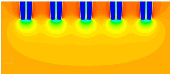
**Figure 4.** Normalised axial velocity contours ( $v_a/V_\infty$ ) in the  $xy$ -plane at a yaw angle ( $\theta$ ) of  $0^\circ$  and with the NREL 5-MW turbine model.
