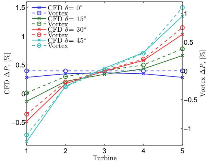
**Figure 8.** Comparison of the percentage changes in the power coefficient for different inflow angles  $\theta$  between CFD-AD simulations and the vortex method. They are presented with respect to two independent  $y$ -axes, but equal scaling. The axes are shifted by 0.4% to each other.
