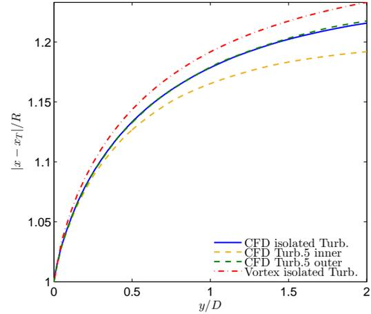
**Figure 10.** Radial wake expansion for an isolated turbine predicted by CFD simulations and vortex method at  $\theta = 0^\circ$ , as well as the inner and outer wake expansion in  $x$  for turbine 5. All turbines had uniform loading.
