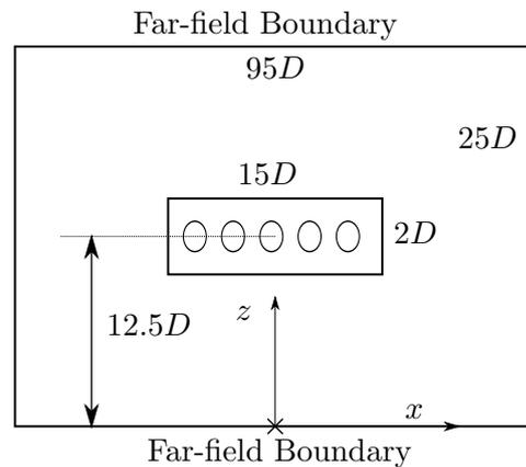
**Figure 3.** Frontal view of the numerical domain.
