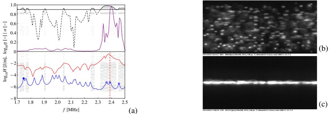
Fig. 2. (a): Behavior of the normalized acoustophoretic mean orientation  $2/\pi\alpha$  (top axes, purple line) as function of the excitation frequency  $f$ . Symbols are the acoustophoretic energy peaks (filled symbol is the optimum according to  $H$ ) and the vertical dashed red line is the optimal working frequency. Purple line is the focusability of the device. (b) & (c): Fluorescence images used in the derivation of focusability parameter.
