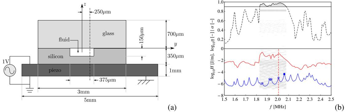
Fig. 1. (a): Schematic of the cross-section of the acoustophoretic device used in the numerical simulations. (b): Behavior of the normalized acoustophoretic mean orientation  $2/\pi\alpha$  (top axes, red line) as function of the excitation frequency  $f$ . Symbols are the acoustophoretic energy peaks (filled symbol is the optimum according to  $H$ ) and the vertical dashed red line is the optimal working frequency.
