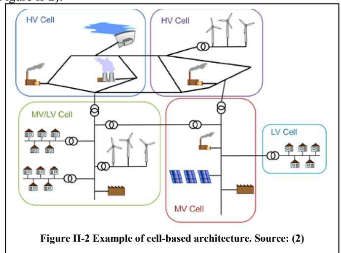
**Figure II-2 Example of cell-based architecture. Source: (2)**
