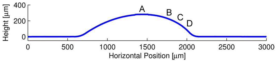
**Figure 2:** Profile of the imprinted surface. The radius of curvature is 1mm, total height is 280  $\mu\text{m}$  and the diameter is 1400  $\mu\text{m}$ . Well defined imprints are obtained at positions A, B and C.
