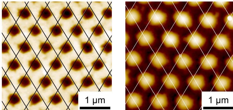
**Figure 3:** An example of unit cell identification to estimate the pitch of the imprinted features. *Left:* AFM image of the PDMS stamp. Mean pitch is 670 nm. *Right:* AFM image of the imprinted surface at the apex (A in Fig. 2). Mean pitch is 820 nm.
