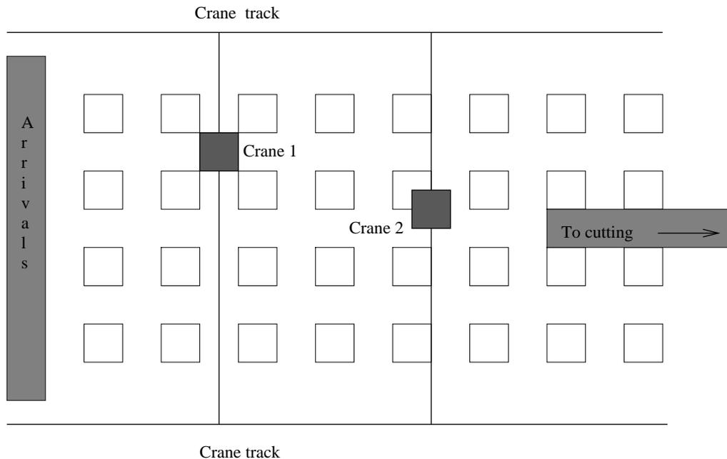
Figure 2. A 4 by 8 steel plate storage with 2 cranes
