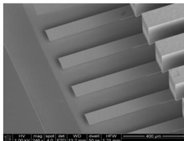
Figure 3. Top view of microcantilever sensors array
