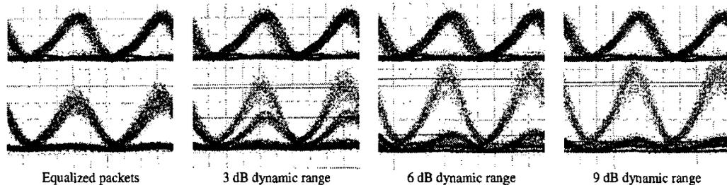
Fig. 3. Eye-diagrams for the input (lower) and the output (upper) for different variations in the packet-to-packet power level.
