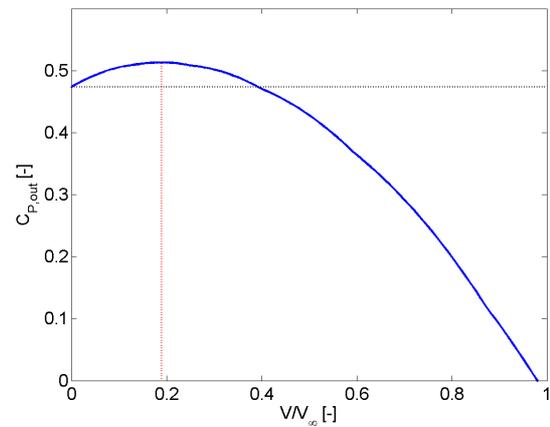
Figure 6: Net output power coefficient  $C_{P,NET}$  as function of vehicle velocity ratio for a vehicle with the key numbers of the vehicle in Section 3.2 and rotor key numbers  $CLCD_{max}=100$  and  $\lambda=5$ .
