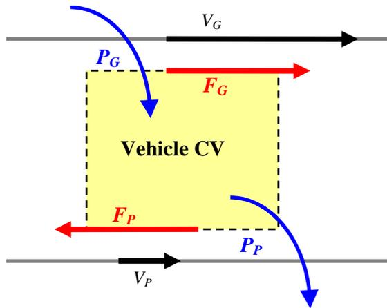
Figure 1: Notation used in investigation of energy conversion mechanisms for vehicles powered by a difference in velocity of two media.
