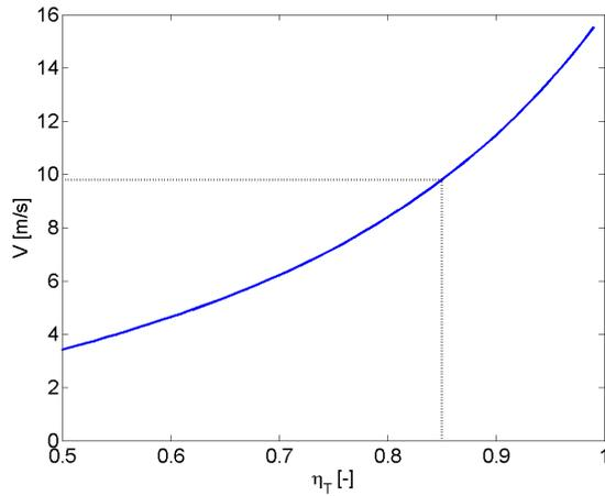
Figure 5: Vehicle velocity with  $V_{\infty}=10\text{m/s}$  free wind. Vehicle velocity is shown as a function of transmission efficiency. Note that each particular point on the curve corresponds to a specific generator rotor design given by the optimization algorithm.
