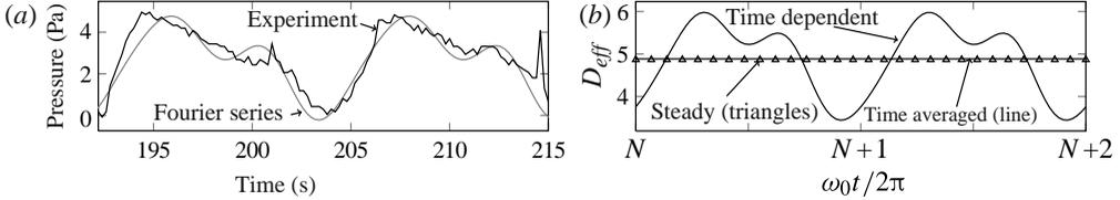
FIGURE 4. (a) Two periods of the measured time-dependent pressure delivered by the peristaltic pump (black) by Skaftø-Pedersen *et al.* (2009) and of the approximate Fourier series ( $|\ell| \leq 3$ ) used in the analysis (grey). (b) Calculated  $D_{eff}(t)$  for the two cycles of the peristaltic pump following period  $N = 10^4$  after the decay of all transients: the Fourier series (black), only the steady component (dashed) and the time-averaged Fourier series (grey).
