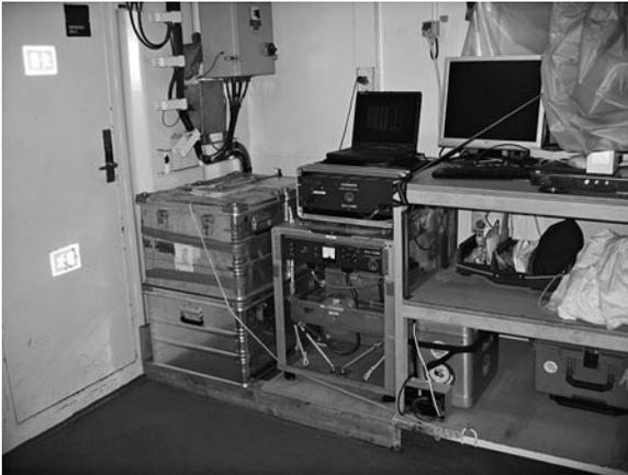
**Fig. 44.2** The LC&R S-38 marine gravity meter in “the hangar”. The LC&R land gravity meter G-867, which was used for the harbour ties, is stored in an aluminium box and strapped to the lower shelf next to the marine meter
