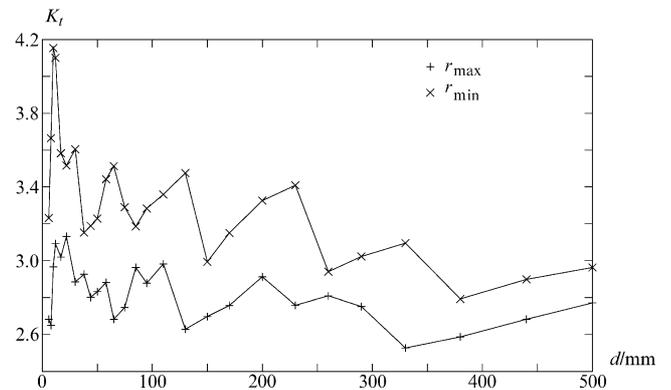
**Fig. 9** The stress concentration factor for the prismatic part of a keyway in pure torsion as a function of the diameter. The different design variables are controlled by DIN 6885. The point corresponds to numerical simulations; these are connected by straight lines
