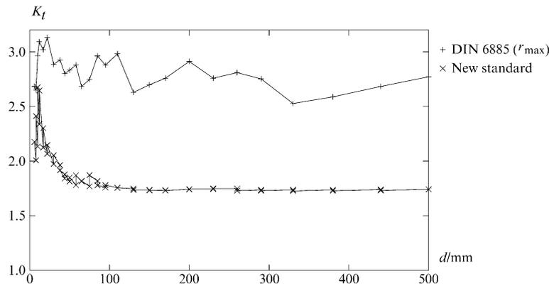
**Fig. 17** The stress concentration factor for the prismatic part of a keyway in pure torsion as a function of the diameter. The top curve is for the DIN 6885 design with the maximum allowable fillet radius. The bottom curve is for the new proposed keyway design. The point corresponds to numerical simulations, which are connected by straight lines
