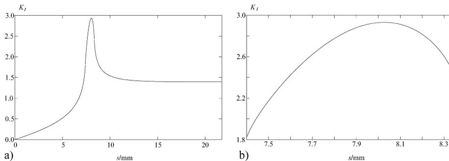
**Fig. 4** The figures are for half the shaft shown in Fig. 2 and show the stress concentration as a function of the arc length. (a) The stress concentration factor along the keyway boundary starting from the external point until the centre point. (b) Stress concentration close up, here only shown along the  $r = 0.6$  mm fillet at the corner. The maximum value is  $K_t = 2.93$ ; with a fillet radius of 0.4 mm, which is also allowed by the standard, the value is  $K_t = 3.32$
