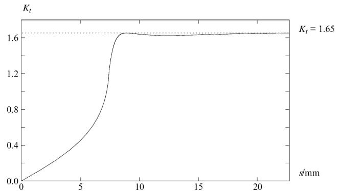
**Fig. 14** The stress concentration as a function of the arc length along the keyway from the external point up to the centre point
