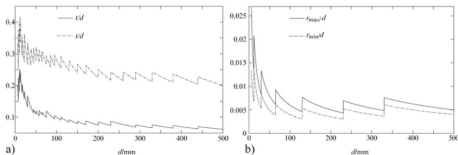
**Fig. 5** (a) The depth ratio  $t/d$  and width ratio  $b/d$  as a function of the shaft diameter according to DIN 6885; (b) the upper and lower limits for the fillet ratio  $r/d$  as a function of the shaft diameter according to DIN 6885
