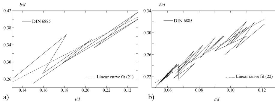
**Fig. 6** (a) The width ratio as a function of the depth ratio for the diameter range  $6 \text{ mm} \leq d \leq 38 \text{ mm}$  according to DIN 6885; the linear curve fit (21) is also shown. (b) the width ratio as a function of the depth ratio for the diameter range  $38 \text{ mm} \leq d \leq 500 \text{ mm}$  according to DIN 6885; the linear curve fit (22) is also shown
