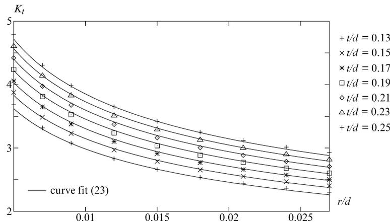
**Fig. 7** The stress concentration factor as a function of the fillet ratio for diameter range  $6 \text{ mm} \leq d \leq 38 \text{ mm}$ . For this diameter range the fillet ratio fulfils  $0.005 \leq r/d \leq 0.027$  and the depth ratio fulfils  $0.13 \leq t/d \leq 0.25$ , according to DIN 6885. The width ratio  $b/d$  is linked to the depth ratio through (21). The numerical calculations are shown by points and the full lines are the curve fit to the data, see equation (23)
