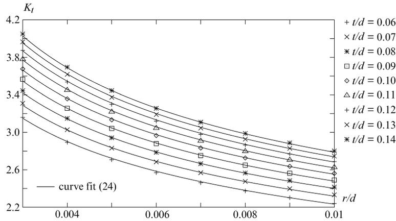
**Fig. 8** The stress concentration factor as a function of the fillet ratio for the diameter range  $38 \text{ mm} \leq d \leq 500 \text{ mm}$ . For this diameter range the fillet ratio fulfils  $0.003 \leq r/d \leq 0.01$  and the depth ratio fulfils  $0.06 \leq t/d \leq 0.14$ , according to DIN 6885. The width ratio  $b/d$  is linked to the depth ratio through equation (22). The numerical calculations are shown by points and the full lines are the curve fit to the data, see equation (24)
