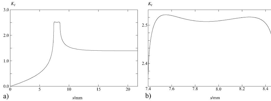
**Fig. 12** The figures are for half the keyway and show the stress concentration as a function of the arc length: (a) the stress concentration factor along the keyway boundary starting from the external point until the centre point; (b) stress concentration close up, here only shown along the super ellipse; the maximum stress concentration factor is  $K_t = 2.53$
