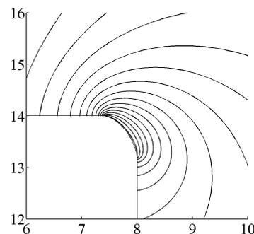
**Fig. 11** Iso lines of largest principal stress for the optimized design
