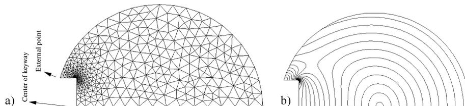
**Fig. 3** The figures are for half the shaft given in Fig. 2. (a) Example of a finite element mesh, the illustrated mesh has 917 elements. The Dirichlet boundary condition (8) is applied to the bottom edge while the Neumann boundary condition (6) is applied to the remaining edges. (b) Iso lines of resulting stress level, indicating the stress concentration at the corner
