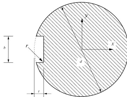
**Fig. 2** Cross-section of prismatic part of parallel keyway, the coordinate system is placed at the shaft axis. The relative dimensions correspond to a  $d = 100$  mm shaft according to DIN 6885-1 [1], ( $t = 10$  mm,  $b = 28$  mm,  $0.4$  mm  $\leq r \leq 0.6$  mm)
