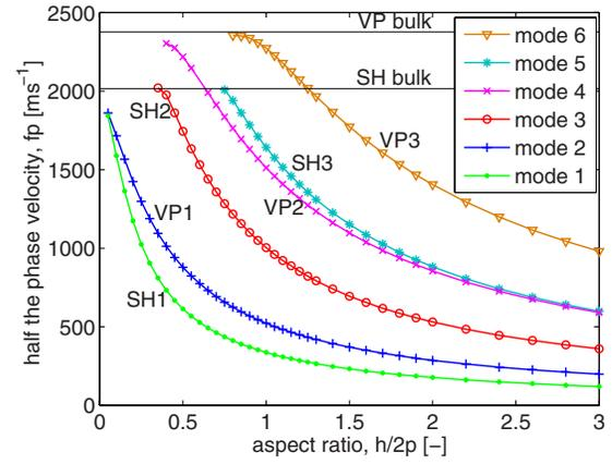
FIG. 2. (Color online) Half of the phase velocity  $fp$  as function of  $h/2p$  for the six first modes for  $kp = \pi/2$ . The polarization types are indicated along with the limits for the bulk waves.
