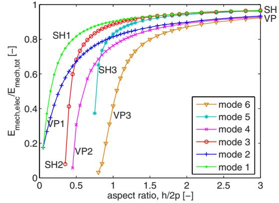
FIG. 5. (Color online) Fraction of mechanical energy in the electrode with respect to the total energy in the structure, as a function of the aspect ratio  $h/2p$  for the first six modes. The propagation constant is  $kp=\pi/2$ . The limit for the SH-type modes is 97% and the limit for the VP-type modes is 93%.
