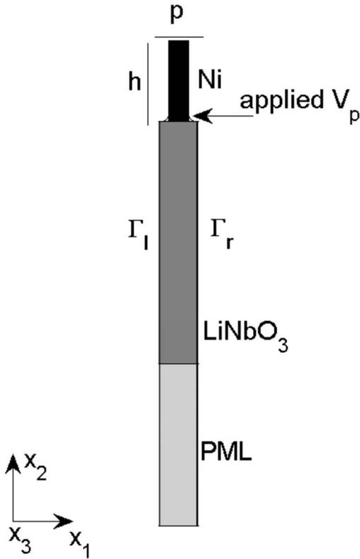
FIG. 1. The geometry of the unit cell with periodic boundary conditions and period  $p$ . The electrode consists of nickel and has the height  $h$ . The substrate is lithium niobate and a PML is placed at the bottom. The electric potential  $V_p$  is applied at the interface between the electrode and the substrate.
