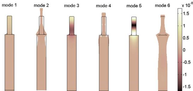
FIG. 4. (Color online) The deflections in the structure for each of the six modes at resonance with  $h/2p=1$  and  $kp=\pi/2$  normalized to  $V_p=1$  V. The deflections  $u_1$  and  $u_2$  are given with an arbitrary scaling factor and  $u_3$  is given by the color bar for all six modes.
