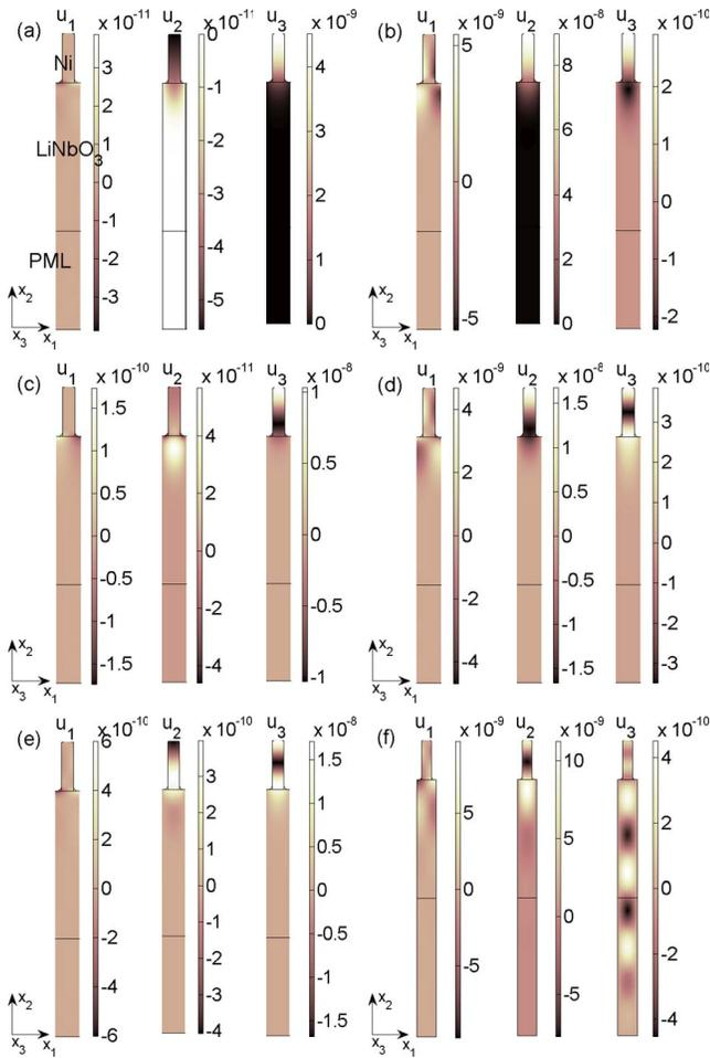
FIG. 3. (Color online) The deflections  $u_1$ ,  $u_2$ , and  $u_3$  at resonance with  $h/2p=1$  and  $kp=\pi/2$ . All deflections are normalized to  $V_p=1$  V. (a) Mode 1, (b) mode 2, (c) mode 3, (d) mode 4, (e) mode 5, and (f) mode 6.
