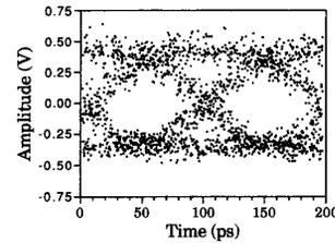
Fig. 3. Eye diagram after preamplifier receiver at BER =  $10^{-9}$ .
