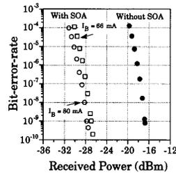
Fig. 2. Measured BER versus received power with and without SOA preamplifier. Bias current to the amplifier is a parameter.
