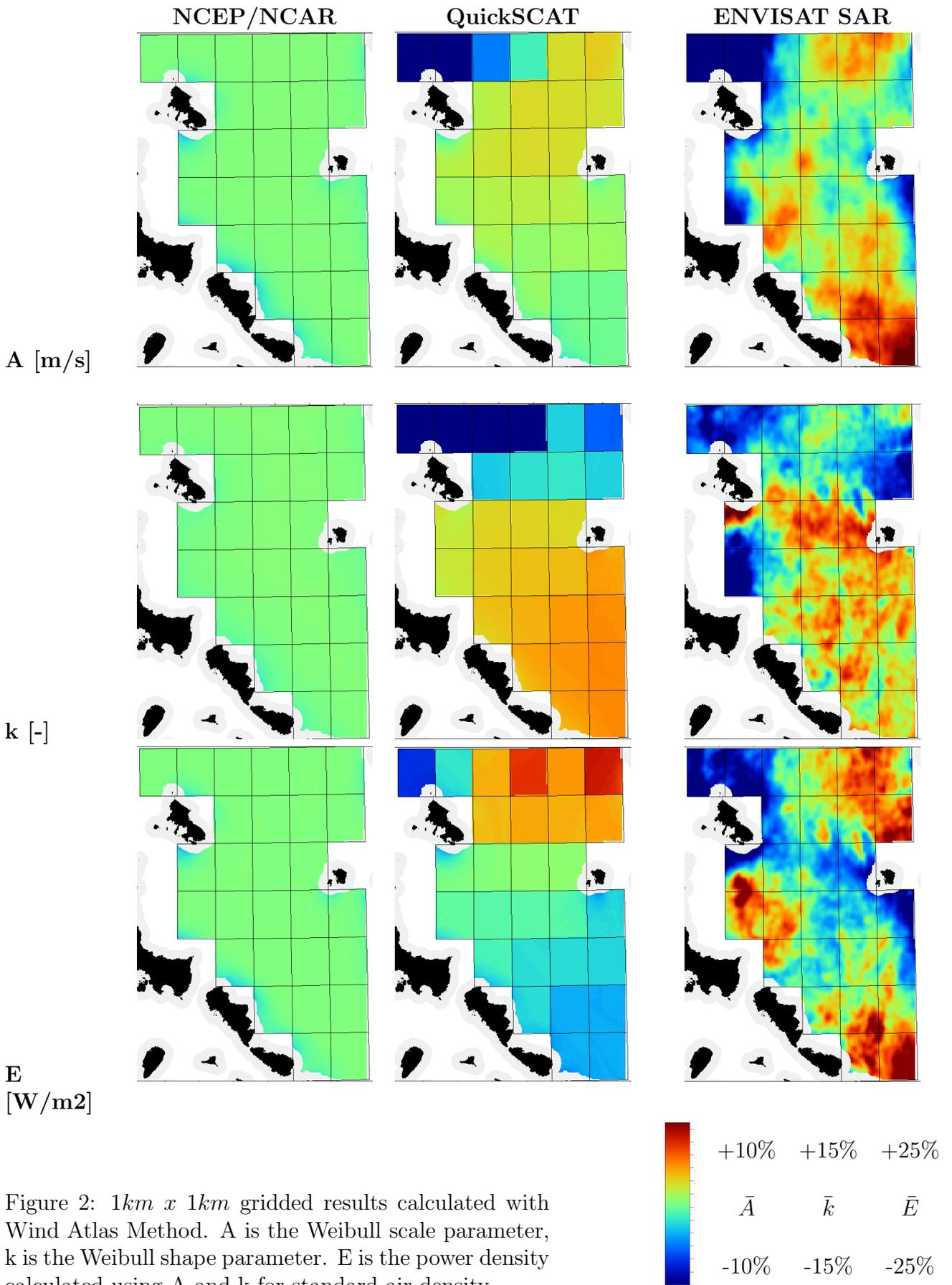
Figure 2:  $1km \times 1km$  gridded results calculated with Wind Atlas Method.  $A$  is the Weibull scale parameter,  $k$  is the Weibull shape parameter.  $E$  is the power density calculated using  $A$  and  $k$  for standard air density.
